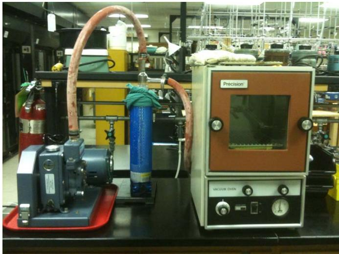
1. Grease vacuum trap using high vacuum silicone grease (white). Attach side arm of trap to back of vacuum oven. Attach top of trap to belt driven vacuum.
