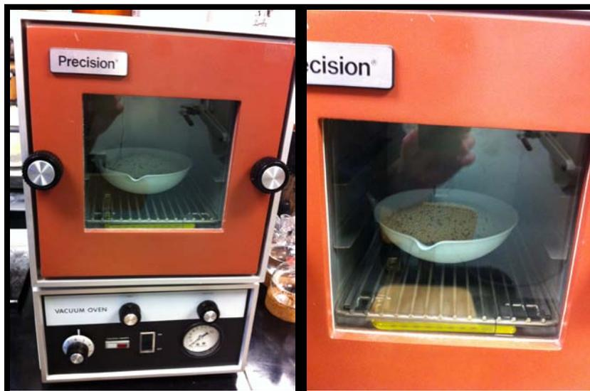
4. Once vacuum has been established and the liq. N<sub>2</sub> trap filled, heat the oven to 190 °C. Leave the molecular sieves under vacuum and at 190 °C for 3 days (72 hours).
