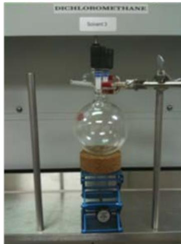
attached & immobilized solvent storage flask under dispenser – side view
