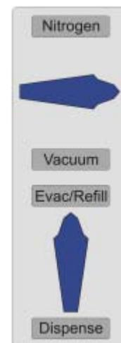
Turn the top valve counterclockwise to the horizontal, **Neutral** position. Make sure the top valve is horizontal and is not on **Vacuum** or **Nitrogen**. The bottom valve should remain in the **Evac/Refill** position. After the third evacuation process is complete, the solvent can be dispensed for use. **DO NOT** remove the collection vessel. Your Schlenk flask is now under a static vacuum and ready to have solvent dispensed to it.
