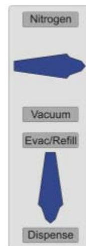
8) After the desired amount of solvent has been dispensed to your Schlenk flask turn the bottom valve slowly counterclockwise to the **Evac/Refill** position.
