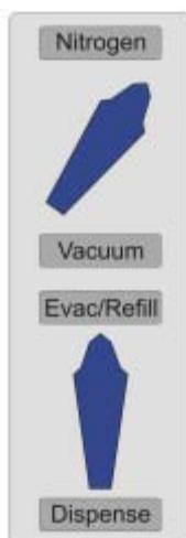
Turn the top valve slowly counterclockwise towards **Nitrogen** and hold it at the 1 o'clock position for 2-5 seconds. This clears the line of solvent and backfills your Schlenk flask with nitrogen gas. Under a positive pressure nitrogen flow carefully remove your Schlenk flask and cap the ground glass joint with a septa.
