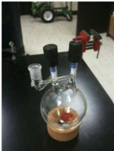
oven dried, solvent storage flask @ 25 °C under vacuum
