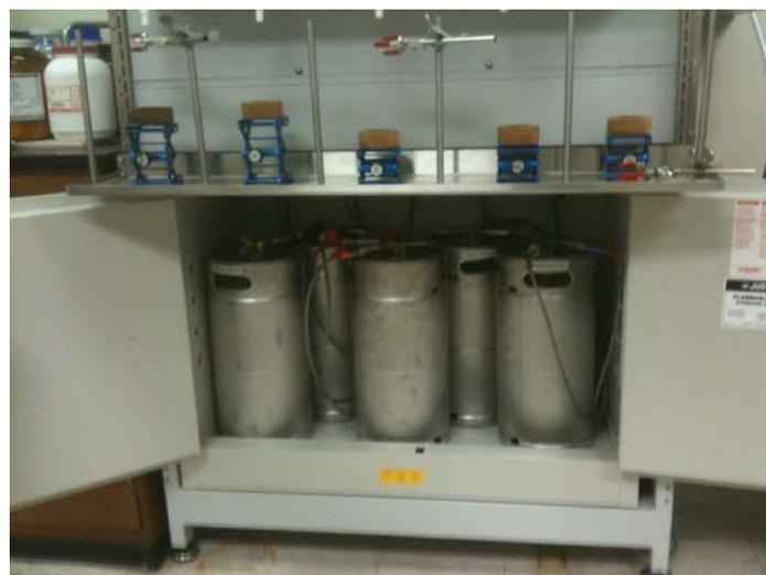
Routine use of the MB-SPS is extremely simple, since the user only needs to operate the color-coded valves located on the front panel of the system. It is important to remember, though, **that all operations must be performed slowly and gradually to avoid rapid pressure changes.**
