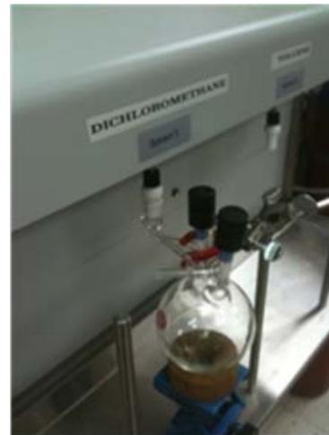
attached & immobilized solvent storage flask under dispenser – top view
