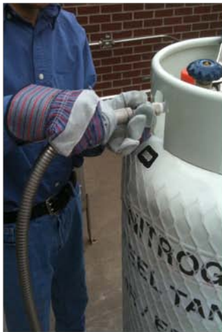
Attach fill hose to the blue liquid valve of dewar. Make sure not to overtighten the connections!!!
