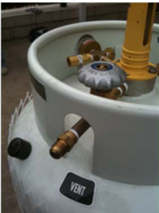
Open the Gray vent valve to release the pressure...
