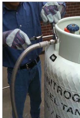
Attach fill hose to the blue liquid valve of dewar. Make sure not to overtighten the connections!!!
