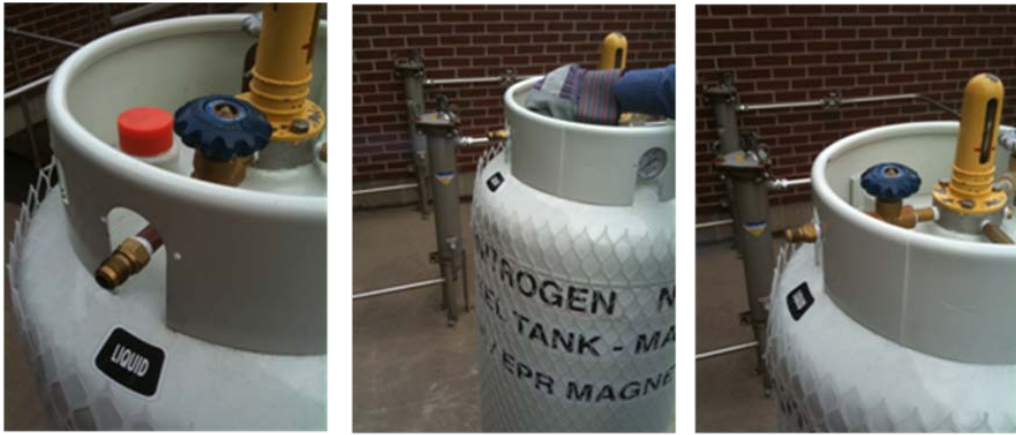
Open the blue liquid vent valve and make sure to not get sprayed by liquid Nitrogen...
