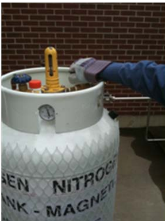
Open the Gray vent valve to release the pressure...
