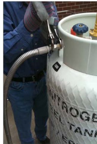
Attach fill hose to the blue liquid valve of dewar. Make sure not to overtighten the connections!!!
