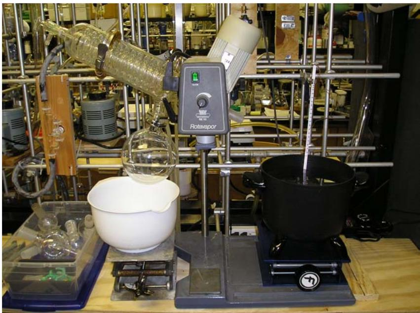
1. Turn chiller unit for rotovap condenser water on. Allow chiller to run for 5-10 minutes before you begin solvent removal on rotovap to allow water temperature to reach 10 °C in condenser.
