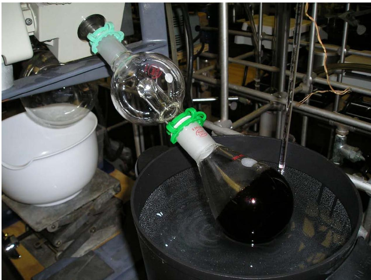
13. Let rotovap run until solvent is pulled off and product is dry. Make sure you see solvent condensing in the rotovap condenser and collecting in flask B.
