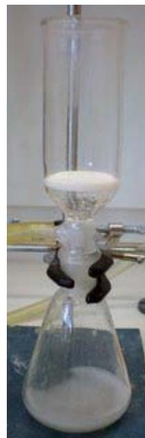
(4) When the ingredients have been cooking away for a minute or so apply a very gentle vacuum briefly. This should be sufficient to suck the sinter dry (See picture above),
